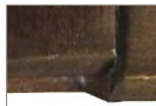
Showing an exposed board at breadboard joint
