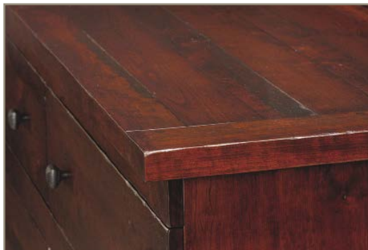
Showing an exposed groove in breadboard
