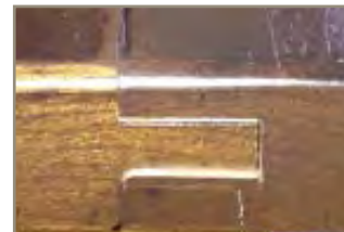
Showing an exposed groove in breadboard
